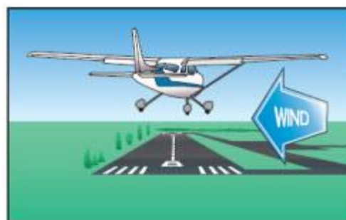
Small Aircraft Crosswind Landing Diagram (faasafety.gov)
